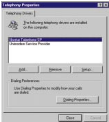
Figure 17. Personal Call Manager: The Norstar Telephony Service Provider installed on our Win95 machine.
