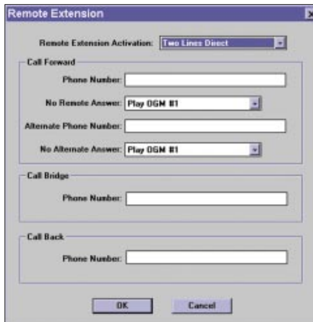
Figure 8. Switchboard: Configuration screen for changing call forwarded number, call back, and other remote extension settings.
