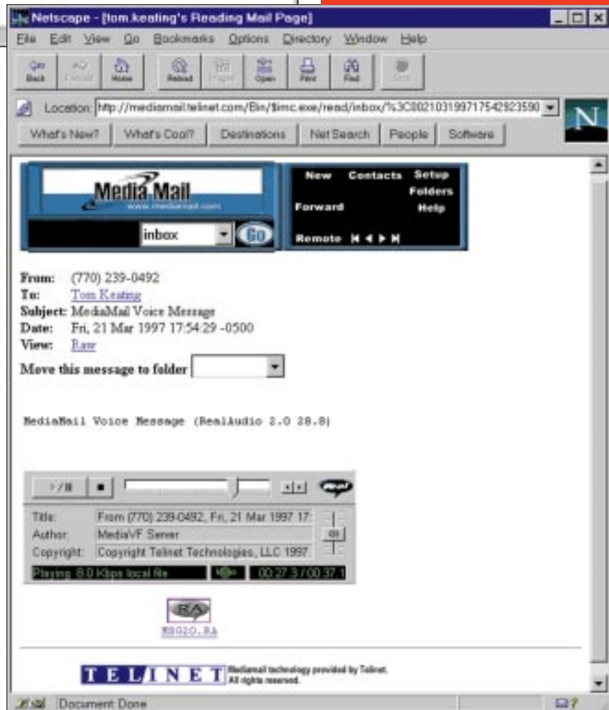
Figure 19. MediaMail: A voice mail message being played and displayed “inline” on the browser.
