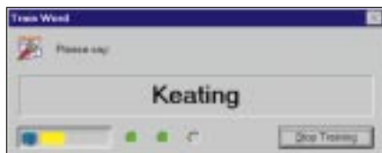
Figure 15. DragonDictate: Training interface to train new words or retrain old ones. The bar on the left indicates how loudly you are speaking into the microphone.
