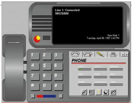
**Figure 7.** PhoneRider: Main GUI showing call control functionality. Here, the display indicates the date and time and notes that line 1 is in use.
