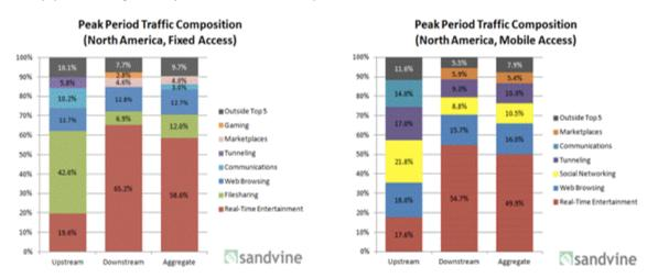
The left figure above shows that 72% of peak period downstream bandwidth consists of large flows comprised of real-time entertainment such as Netflix, Hulu, YouTube, etc. including file sharing. The figure on the right shows that 55% of peak period downstream bandwidth consists of large flows.<sup>[2]</sup>
