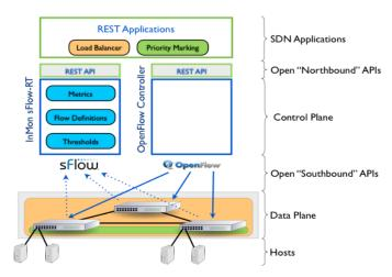
Standard sFlow enabled on the switches and routers provides a continuous stream of measurement data to InMON sFlow-RT, which provides real-time detection and notification of elephant flows to the SDN application. The SDN application selects a marking action and instructs the SDN controller to push the action to the selected switches (for example, using standard OpenFlow rules to assign a selected queue for traffic associated with the large flows).
