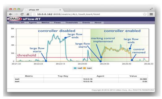
The diagram shows that implementing traffic engineering using OpenFlow and standard sFlow based analytics is shortening significantly the amount of time required to implement controls while guaranteeing uninterrupted services to short lived flows.
