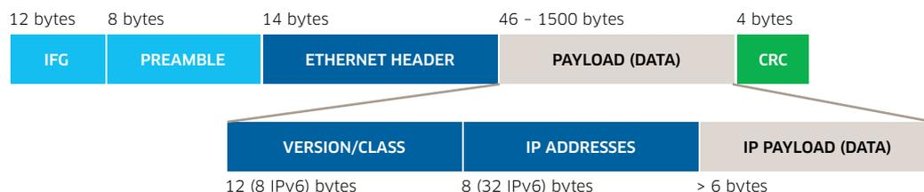
The first two fields, Interframe Gap (IFG) and preamble, are not transmitted over the air and therefore not needed in a microwave transmission, so automatically 20 bytes can be entirely eliminated per Ethernet frame.
