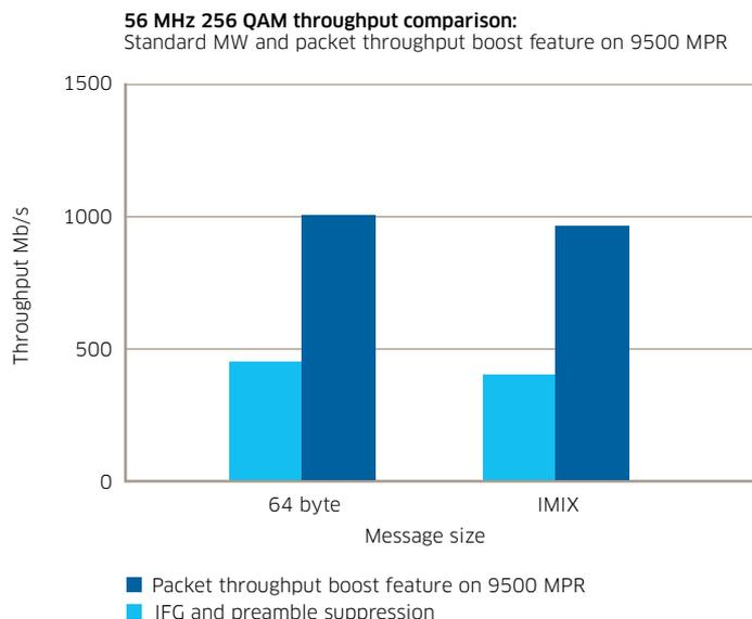
The light blue bar represents microwave with standard 20 byte suppression, and the dark blue bar represents throughput capacity gained with Alcatel-Lucent packet throughput boost feature, which also includes IFG and preamble suppression. As you can see, there is significantly more throughput gained using packet throughput boost header compression when compared to the standard microwave gains achieved with IFG and preamble suppression.
