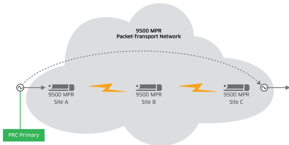
To support IEEE 1588v2 PTP[2] time and frequency[3] synchronization distribution, the 9500 MPR supports patented fragmentation and interleaving techniques to guarantee a synchronization mask of 16 ppb.
