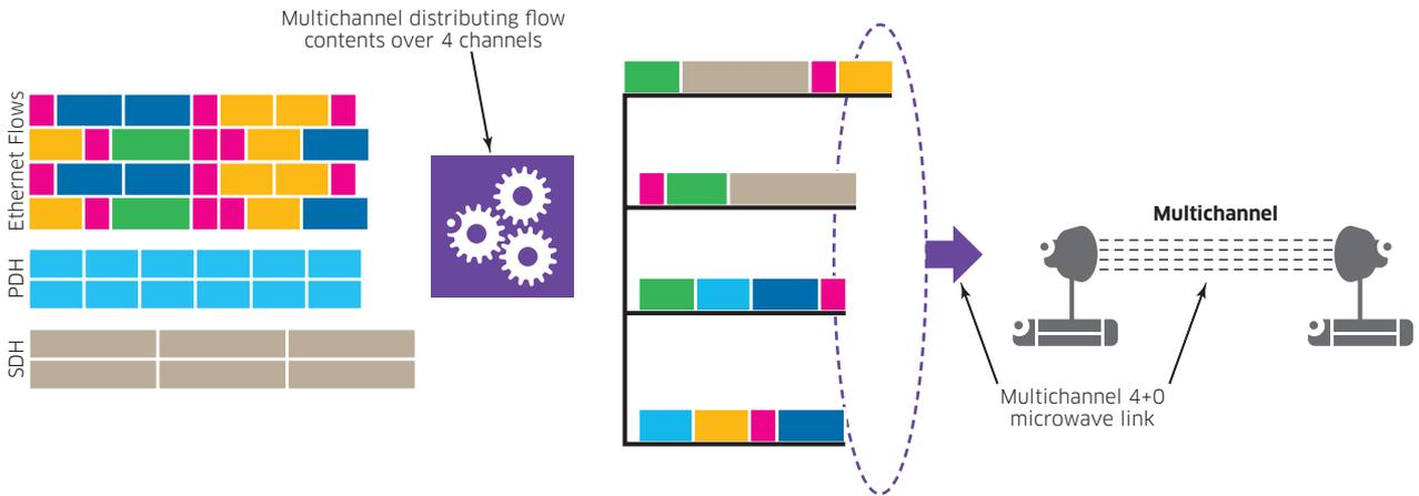
Because the Alcatel-Lucent 9500 MPR transports all services in a packet format (that is, traditional TDM and ATM services are packetized) it can take full advantage of an adaptive modulation aware multichannel capability:
