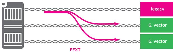
This paper describes and offers solutions to operational challenges created by two specific mixed deployment scenarios. In the first scenario, lines sharing the same binder are connected to digital subscriber line access managers (DSLAMs) from different operators using a local-loop unbundling (LLU) process. Shown in Figure 2, this type of shared deployment can increase FEXT and degrade performance for both operators.
