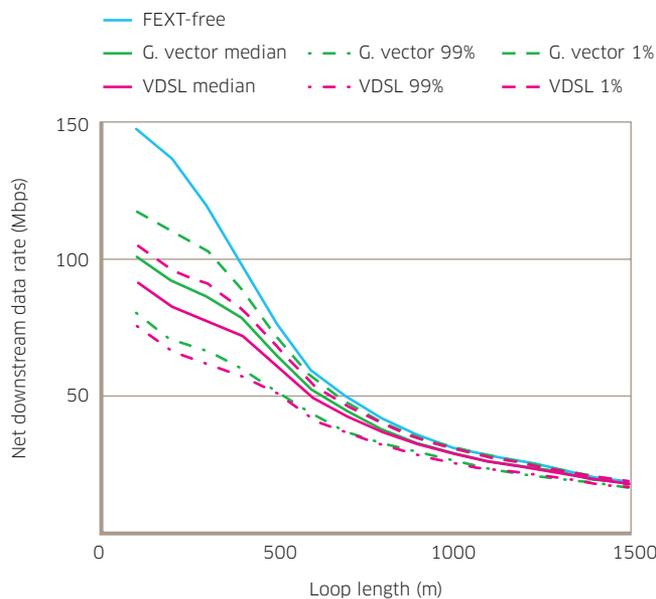
It is notable that the performance drop that legacy VDSL2 lines create on vectored lines is similar to that created when multiple operators deploy vectored lines in an LLU context. These performance drops make it difficult for operators to simultaneously manage vectored and non-vectored lines.
