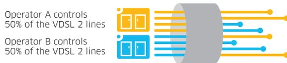
In the second scenario, legacy VDSL2 and vectored lines coexist in the same binder. This situation occurs when an operator introduces vectoring in increments. The challenge for the operator is to ensure that the combination of line types does not offset or eliminate the performance gains offered by the vectored lines.
