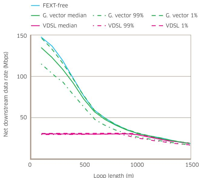
When the extra SNR capacity is used to reduce the transmitted power, vectored line performance improves significantly, averaging close to FEXT-free performance.
