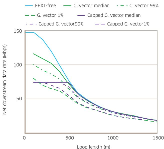
In a scenario with two vectored groups, the ISB approach achieves the same median rates as the *maxPSD* approach used by Algorithm 1. The difference between the median rate achieved through *maxPSD* and ISB is below 0.2 Mbps at every rate–reach point. In addition, the ISB approach does not guarantee more reach than the *maxPSD* approach. At the 99th percentile, the difference in the median rate achieved through *maxPSD* and ISB remains below 1 Mbps for every rate–reach point.
