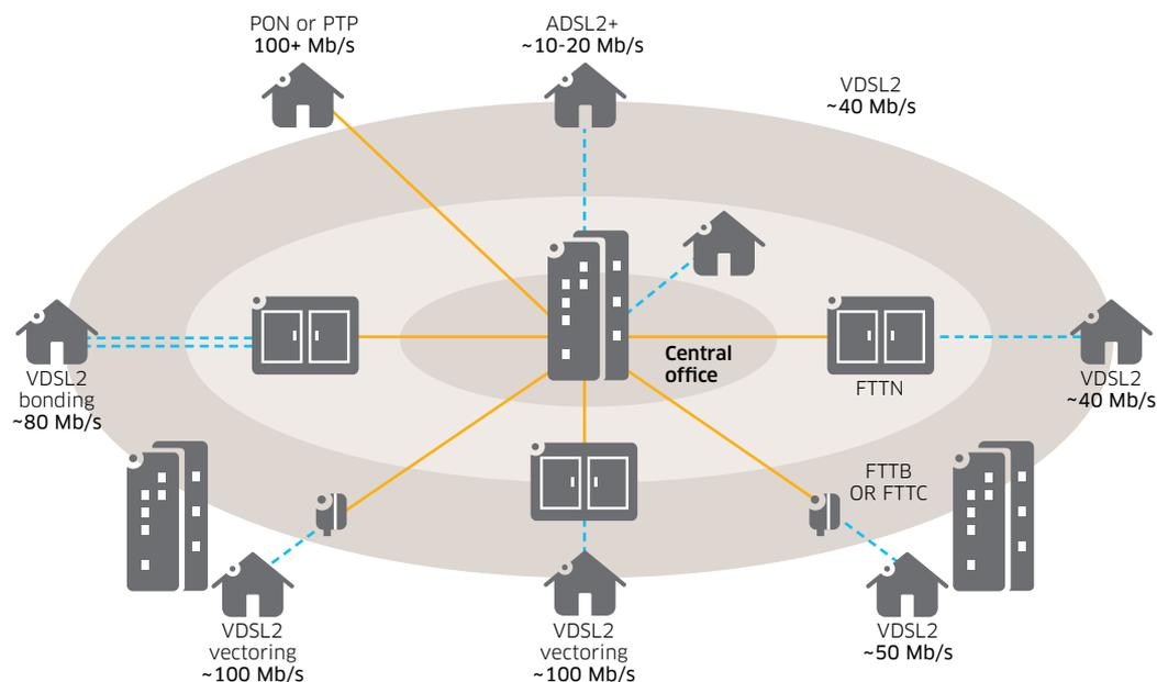
In addition, with VDSL2 bonding the possible distance from the DSLAM for a particular bit rate increases. This allows service providers to offer advanced services to subscribers who might otherwise remain out of reach for those services. Two-pair VDSL2 bonding can also double the attainable bit rate at the same distance from the DSLAM.
