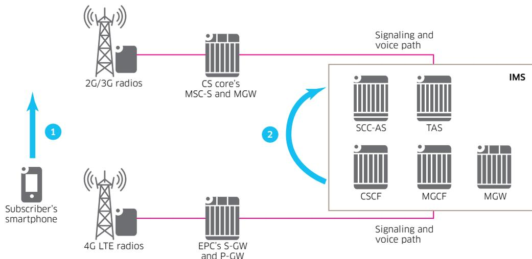
On the IMS side, the procedure for handing over a VoLTE call from 4G LTE to the 2G/3G CS core comprises the following steps:
