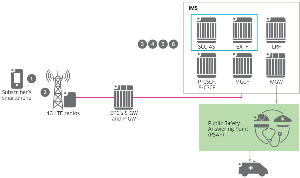
Focusing on SR-VCC, emergency calls must be supported even if the subscriber moves out of 4G LTE coverage during the call. The process for this support is similar to that of the SR-VCC procedure on the IMS side (see Figure 3, steps 1 and 2), except the SCC-AS role in a normal SR-VCC handover is instead provided by the EATF (see Figure 5).
