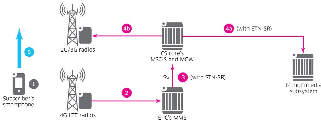
On the mobile side, handover of a call from 4G LTE to the 2G/3G CS core comprises the following steps:
